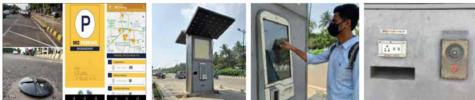
Figure 15: On-ground parking occupancy sensors (left), Mo Parking app interface (right) (BSCL, 2022)
