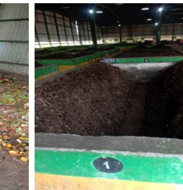
Figure 10: Shredded waste transferred to compost tubs Source: Author
