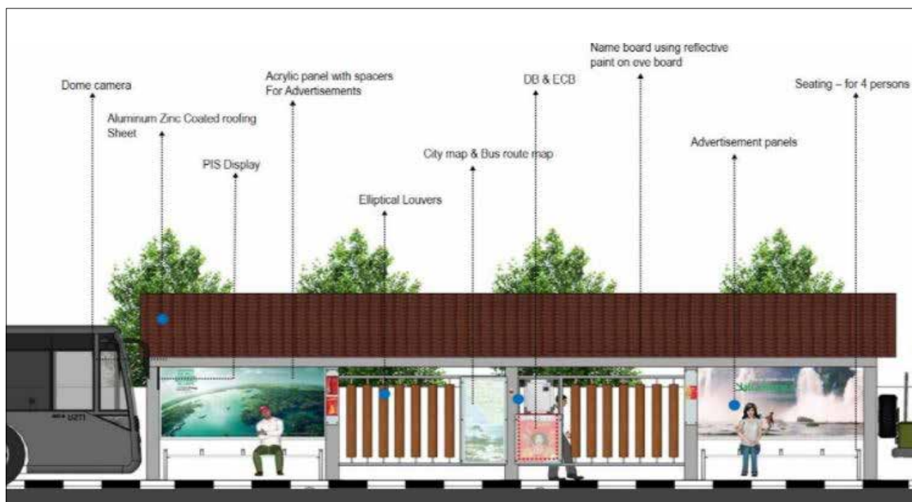
Figure 11: Model Smart Bus stop – 12mX1.8 m module Source: Smart city Trivandrum website
